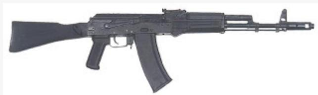
AK-74M assault rifle. Note the complete lack of wooden parts. Click on image to enlarge.
